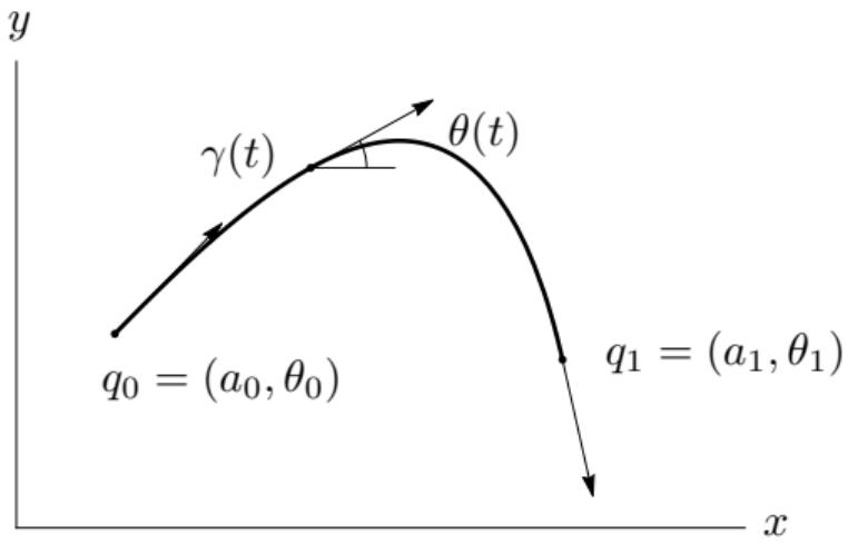
$$\begin{aligned}\dot{x} &= \cos \theta, & q = (x, y, \theta) \in \mathbb{R}^2 \times S^1, \\ \dot{y} &= \sin \theta, & u \in \mathbb{R}, \\ \dot{\theta} &= u, \\ q(0) &= q_0, & q(t_1) = q_1, \\ t_1 &= l \text{ длина стержня,} \\ J &= \frac{1}{2} \int_0^{t_1} u^2 dt \rightarrow \min.\end{aligned}$$
