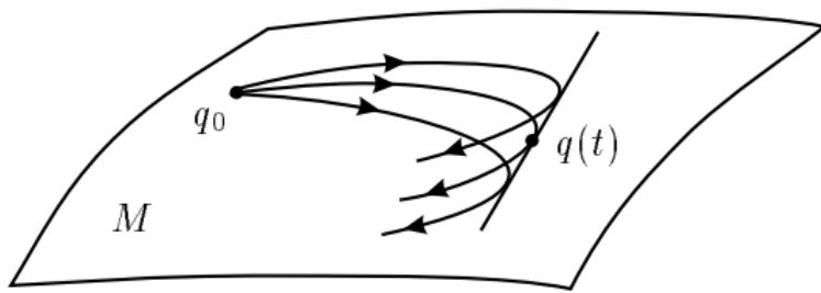
**Figure:** At conjugate point extremal trajectories have envelope
