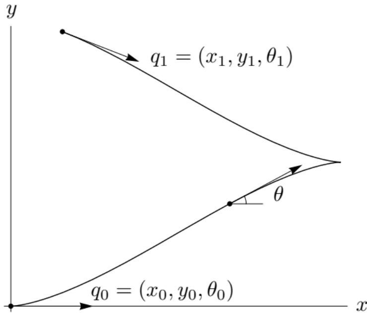
$$q(0) = q_0, \quad q(t_1) = q_1, \quad I = \int_0^{t_1} \sqrt{\dot{x}^2 + \dot{y}^2 + \dot{\theta}^2} dt \rightarrow \min$$
