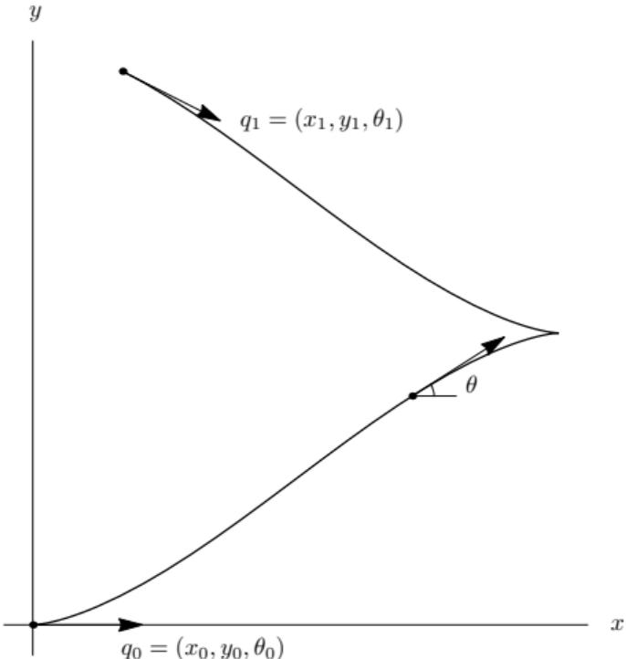
$$\begin{aligned}\dot{x} &= u \cos \theta, & q = (x, y, \theta) \in \mathbb{R}^2 \times S^1, \\ \dot{y} &= u \sin \theta, & (u, v) \in \mathbb{R}^2, \\ \dot{\theta} &= v, \\ q(0) &= q_0, & q(t_1) = q_1, \\ I &= \int_0^{t_1} \sqrt{u^2 + v^2} dt \rightarrow \min.\end{aligned}$$
